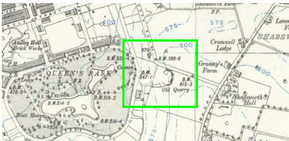
Figure Eight – Plan Showing Historic Quarry Workings
